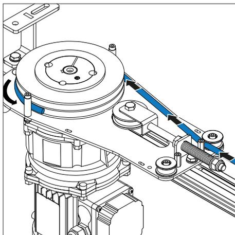
2. Thread the rope into the guide pulley and proceed around the lower groove of the drive sheave.
