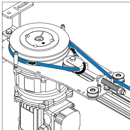
3. Turn around the tensioner idler pulley and then into the upper groove of the drive sheave.
