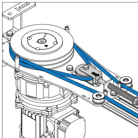
6. After a few cycles the spring mechanism will extend to compensate the elasticity of the rope.
