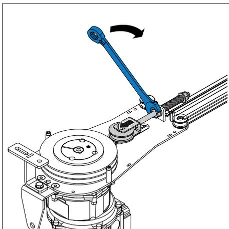
1. Using a 17 mm wrench, compress the spring mechanism.
