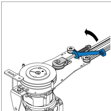
5. Loosen completely the threaded stud with the wrench.
