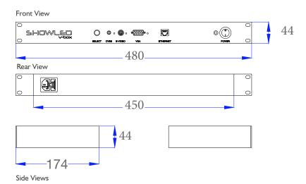
Typical Depth with connectors - 220mm
